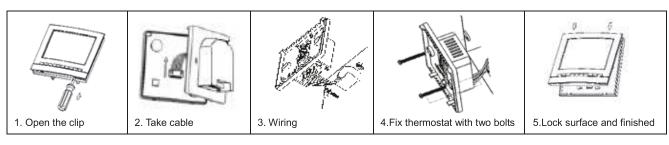
Note: Be sure to connect all the wires as per the wiring diagrams and keep it away from water, mud and other material so as to prevent the unit being spoiled!
